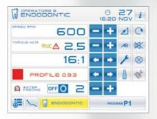
In endodontics mode, the Full Touch software sets combined torque/speed values according to the selected file by drawing on data in preloaded library files.
