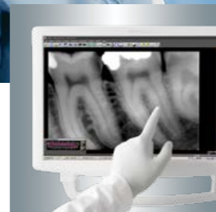
19" LED Monitor CE 93/42 certified, the 16:9 monitor comes complete with a lead for connection to the PC. LED light sources ensure outstanding contrast and brightness. A touch-screen version is also available.
